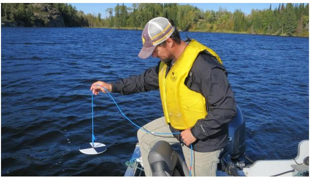
Figure 2 – Lowering of Secchi disk
